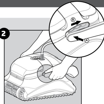
The robot's handle should be adjusted and locked diagonally in order to ensure optimum cleaning results.
