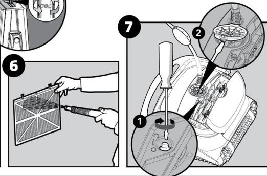
Dismantle the impeller cover and clean around the impeller housing, then reassemble.
